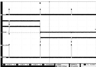
Figure 10. Mode Transition from 1.5x to 1x Mode Using PWM Control (V<sub>CATHODE</sub> Ramp Down) at 2% Duty Cycle
