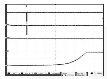
Figure 15. Linear Dimming via I $^2$ C Interface, V<sub>IN</sub>=3.6V, I<sub>LEDx</sub>=20mA, and t<sub>RAMP</sub>=6.4ms
