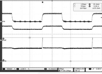
Figure 12. Line Transient Response in 1.5x Mode, V<sub>IN</sub>=2.7V - 3.3V, I<sub>LED</sub>=20mA
