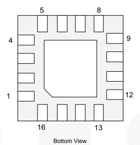
Figure 3. UMLP-16, 0.5mm Pitch, 3mm x 3mm
