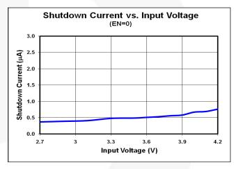
Figure 7. Shutdown Current vs. Input Voltage
