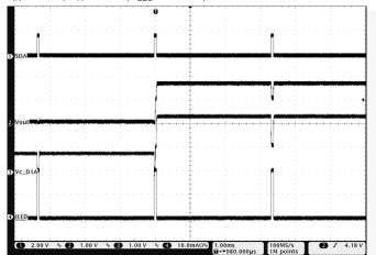
Figure 9. Mode Transition from 1x to 1.5x Mode Using PWM Control ( $V_{CATHODE}$  Ramp Up) at 2% Duty Cycle
