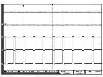
Figure 16. PWM Dimming,  $V_{\text{IN}}$ =3.6V,  $I_{\text{LEDx}}$ =20mA, and EN=1kHz with 20% Duty Cycle
