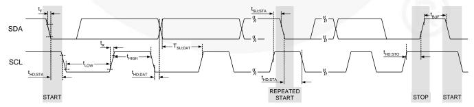
Figure 18. I<sup>2</sup>C Interface Timing for Fast and Slow Modes
