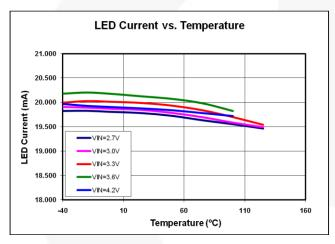
Figure 6. LED Current Variation vs. Temperature
