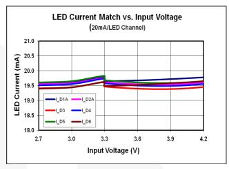
Figure 5. LED Current Match for all 6 LED Channels at  $I_{\text{LED}}$ =20mA.
