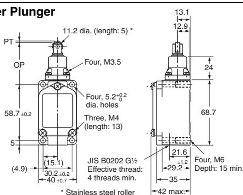
Note: Unless otherwise indicated, a tolerance of ±0.4 mm applies to all dimensions.
