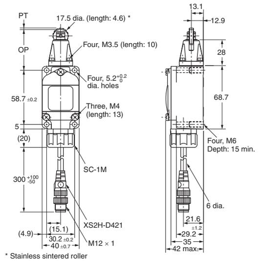
Note: 1. Unless otherwise indicated, a tolerance of  $\pm 0.4$  mm applies to all dimensions.
