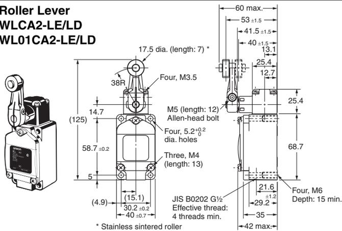
Note: Unless otherwise indicated, a tolerance of  $\pm 0.4$  mm applies to all dimensions.
