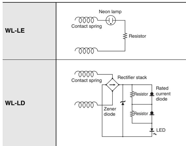
Note: 1. The indicator cover cannot be replaced on the molded terminals. In all cases the indicator does not light when the load is ON.
