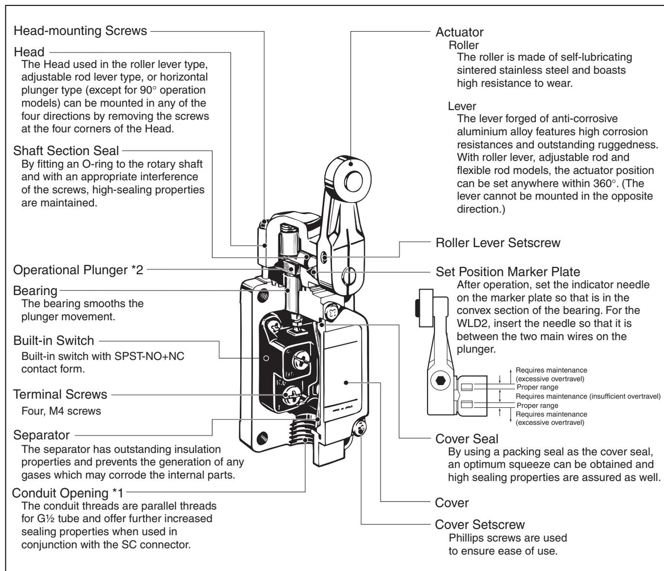
\*1. The display for conduit threads has changed from PF $\frac{1}{2}$  to G $\frac{1}{2}$ , according to revisions of JIS B 0202. This is only a change in the display, so the thread size and pitch have not changed. (Conduit threads Pg 13.5 and  $\frac{1}{2}$ -14NPT are also available.)
