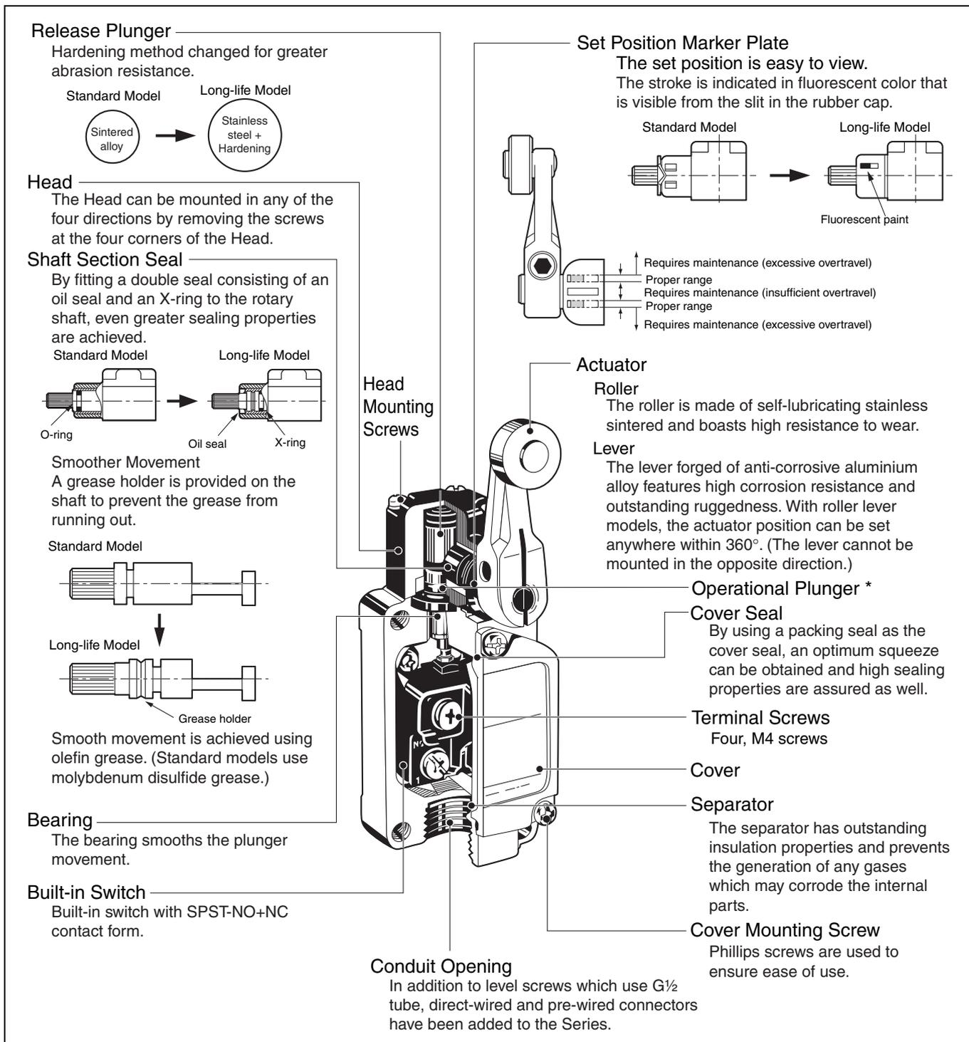
\* By changing the direction of the operational plunger, any one of the three operational directions (both sides, left, or right) can be selected.
