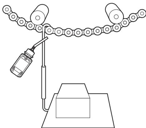
Pallet Detection in Arc Welding Lines
