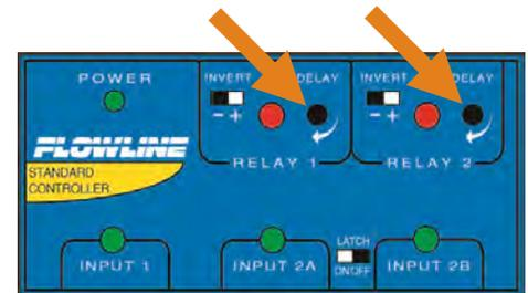
**Note:** The delay has stops on each end of its 270° rotation.
