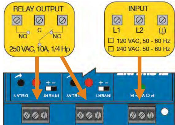
**VAC POWER INPUT WIRING:**
