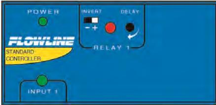
**LC41 series faceplate:** 2 sensor inputs, 1 relay output. The relay included is a latching relay.
