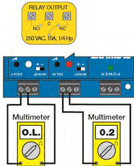
The relay contacts are true dry contacts with no voltage sourced within the relay contacts. To test, connect a Multimeter set to read Ohms.
