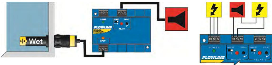
To do this, connect the hot lead of the alarm to the NC side of the relay terminal of the controller. If power is lost, the relay will be de-energized, and the alarm will sound (if there is still power to the alarm circuit itself).
