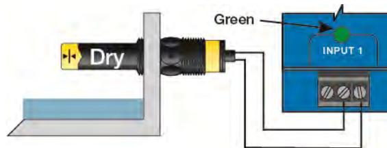
In this state, the relay can be energized with Invert in the OFF setting or can be de-energized with Invert in the ON setting.
