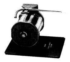
Keeps working area tidy and reduces solder wastage. The solder wire is led from the solder dispenser through a guiding tube. The SD-1000 can be positioned for the soldering job in such a way that the hands of the operator are free for the soldering iron and the component to be soldered.
