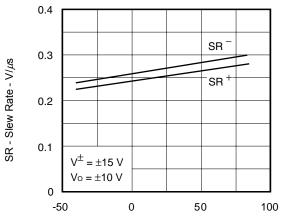
T<sub>A</sub> - Operating Ambient Temperature - °C
