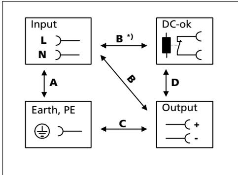
B\*) When testing input to DC-OK ensure that the max. voltage between DC-OK and the output is not exceeded (column D). We recommend connecting DC-OK pins and the output pins together when performing the test.
