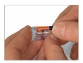
1. Strip the conductor 11mm (4mm² version) or 13mm (6mm² version).
