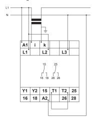
Connected 3~ 400V with power module 400V a.c. with fault latch and current transformer  $I_{\rm N}\!\!>\!\!12A$
