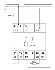
Connected 1~ 230V with power module 230V a.c. without fault latch but with current transformer  $I_{\rm N}{>}12{\rm A}$
