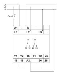
Connected 3~ 400V with power module 400V a.c. with fault latch and temperature monitoring sensor  $\mathbf{I_{N}} \!\!<\! \! \mathbf{12A}$
