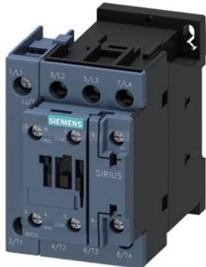
contactor AC-1, 40 A, 400 V / 40 °C, 4-pole, 400 V AC, 50 Hz, auxiliary contacts: 1 NO + 1 NC, screw terminal, size: S0
