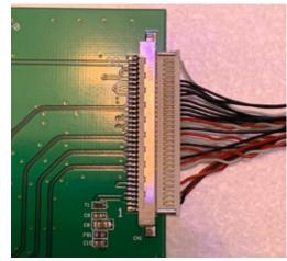
The connection should look like this when the connector is connected correctly.
