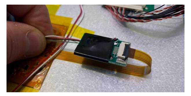
Insert the USB mini connector into the adapter board and connect to your PC
