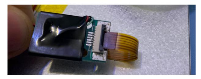
Close the flap to secure the FFC tail
