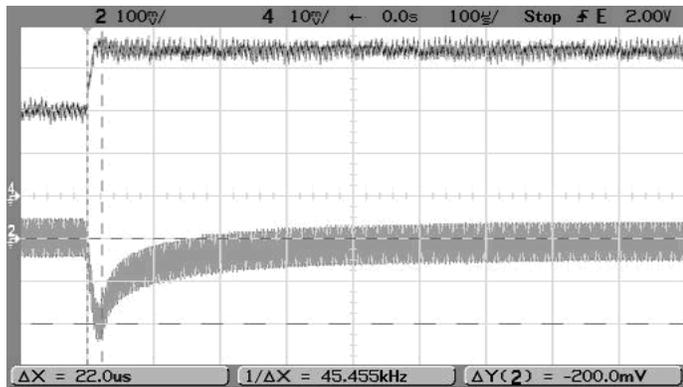
Step Load Transient Response (VIN=24V, Vout=12V, Cload=0, Iout=3A to 1.5A)
