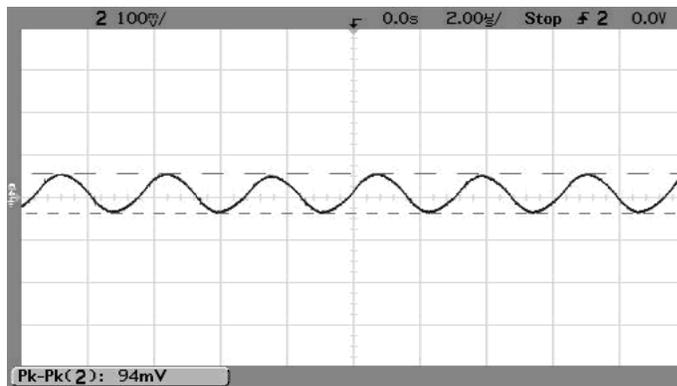
Step Load Transient Response (VIN=24V, Vout=12V, Cload=0, Iout=1.5A to 3A)
