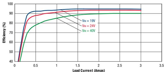
Efficiency vs. Line Voltage and Load Current @ +25°C
