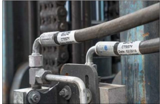
Helatag 1232 – self-laminating labels with good resistance to alcohol and hydraulic oils.
