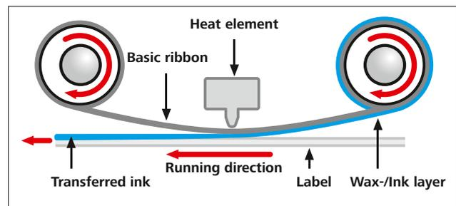
Heated dots strike a special colour ribbon, the thermal transfer film, which transfers liquefied colour ink at exactly that point onto the backing material (labels, tubes, rating plates). Our modern printers use what is known as "thin film technology", in which the very brief liquid phase of the ink produces faster print speeds and better and more precise images than with the "thick film technology" formerly used.
