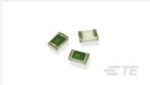
TE Part #2-2176091-6 RP 2A 0.25W 105R 0.1% 25PPM 1K RL
