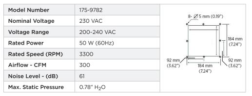
\* Note: Airflow data is for the fan without the louvered filter attached. Calculations indicate that up to a 40% reduction (~ 180 CFM) in fan airflow is possible with LFG unit installed.
