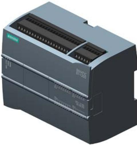
SIMATIC S7-1200, CPU 1215C, CPU COMPATTA, DC/DC/DC, 2 PORTE PROFINET, I/O ONBOARD: 14 DI 24VDC; 10 DO 24VDC; 0,5A; 2 AI 0-10V DC, 2 AO 0-10V DC, ALIMENTAZIONE: DC 20,4 - 28,8 V DC, PROGRAMMA/MEMORIA DATI 100 KB
