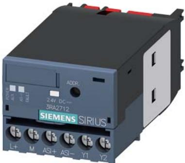
function module for AS-i, direct start, screw terminal, can be snapped on at the front on communication-capable contactor 3RT20.....-0CC0
