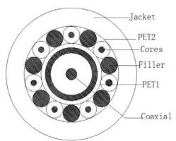
Cable Marking: 7 core + 75  $\Omega$  coaxial cable 001M...100M
