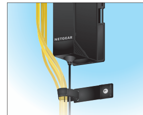
Strap the cables to the wall
