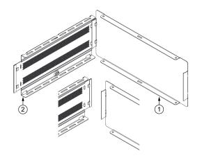
Assemble Side Frame to Front Rear Panel.
