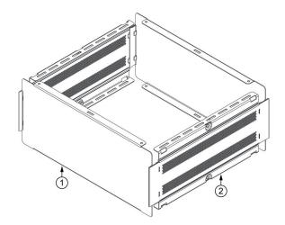
2. Complete Side Frames and Front Rear Panel assembled.
