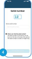
Enter the Serial Number of the Meter to Pair the Meter with the App.
