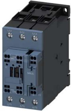
power contactor, AC-3e/AC-3, 80 A, 37 kW / 400 V, 3-pole, 20-33 V AC/DC, 50/60 Hz, with integrated varistor, auxiliary contacts: 1 NO + 1 NC, main circuit: screw terminal, control and auxiliary circuit: spring-loaded terminal, size: S2, communication-capable
