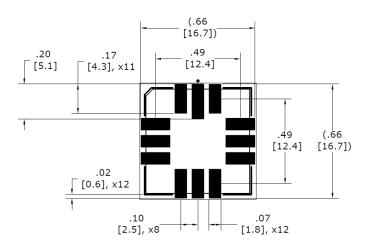
PC board solder pad layout and dimensions
