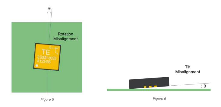
Both types of misalignment errors result in incorrect output voltages for vibration amplitude. The output error will be proportional to the cosine or 1-cosine of the error angle  $\theta$ .
