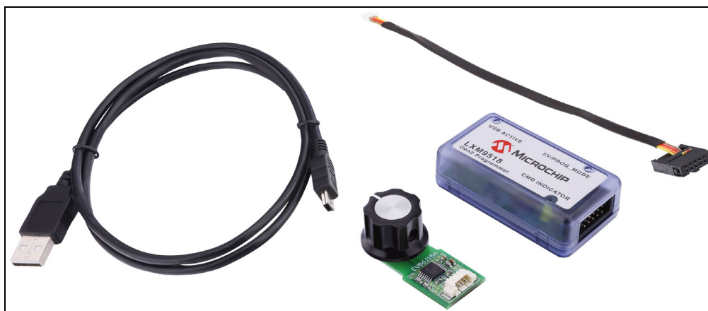
FIGURE 1-2: LX34311 120 Degree Rotary Kit (EV02D18A).
