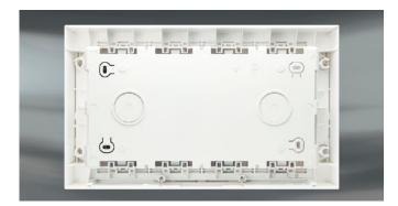
The boxes are linked in a very simple way: the side is cut with scissors, the connection pieces that the box has inside are rotated and these are joined to the other box by simple pressure. This provides a perfect connection that does not alter the design of the box. (Figure 1).
