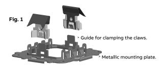
Once the claws are assembled, place the screwdriver in the mounting plate to level it and mount it correctly in the box.
