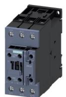
power contactor, AC-3e/AC-3, 65 A, 30 kW / 400 V, 3-pole, 20-33 V AC/DC, 50/60 Hz, with integrated varistor, auxiliary contacts: 1 NO + 1 NC, screw terminal
