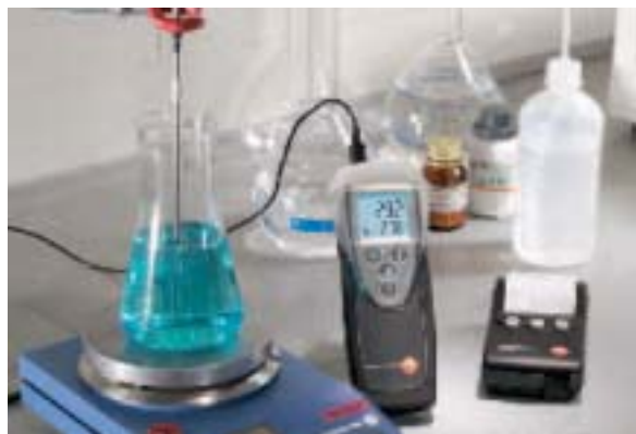
Precise temperature measurement in industry and laboratories with measurement data printing on location
