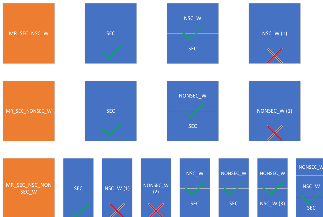
Figure 14-2. Splittable Main Regions Configurations
