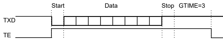
Figure 36-19. Example of TE Drive with Guard Time
