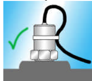
Fig 7: Removing connection strain by anchoring cable to the accelerometer
