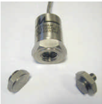
Fig 4: Transducer with Quickfit base showing adhesive and threaded adaptors
