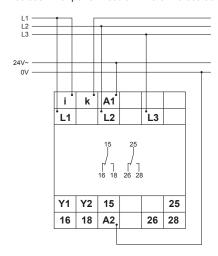
Connected  $3\sim 500V$  with power module 500V a.c. with fault latch  $I_N$ <16A
