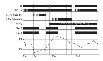
Example: Window function (WIN) - Resetting the fault latch by pressing the reset-key
