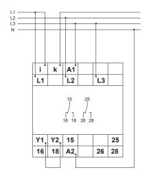
Connected 3~ 400/690V with power module 400V a.c. with fault latch and current transformer  $\rm I_{\rm N}{>}16A$
