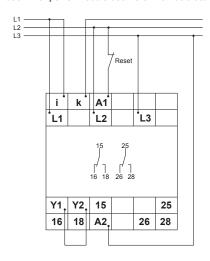
Connected 3~ 230/400V with power module 230V a.c. with fault latch I<sub>N</sub><16A
