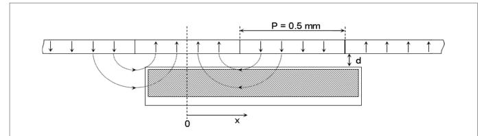
Fig. 1: Arrangement of sensor and magnetic scale. In this example the sensor moves in the x-direction along the fixed scale. The illustrated chip length does not correspond to the actual length relative to the pole pitch.
