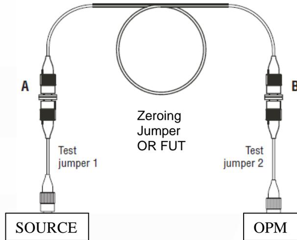
**Measure the Loss of a Fiber Link and Include the Connector Losses:**
