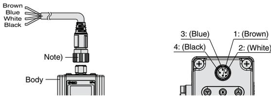
Note) The cable is also available in a right angle type. A right angle type connector is attached facing left (toward the SUP port). Do not attempt to rotate, as the connector does not turn.
