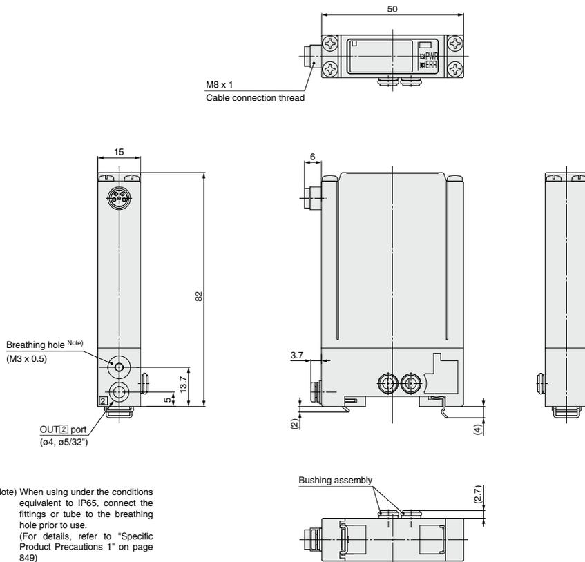
Note) When using under the conditions equivalent to IP65, connect the fittings or tube to the breathing hole prior to use.
