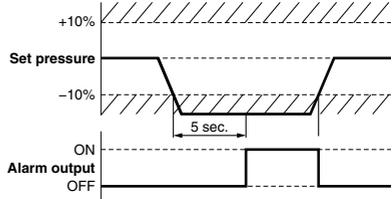
Figure 2. Relationship between output pressure and alarm output
