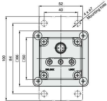
Note) Do not attempt to rotate, as the cable connector does not turn.
