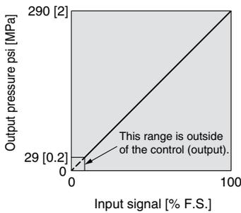
**Fig. 1. Input/output characteristics chart**
