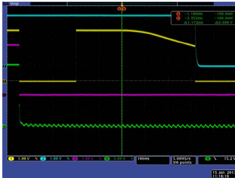
Figure 7. NCN5150 Shutdown Sequence
