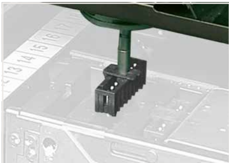
THR male headers for reflow soldering in SMT applications
