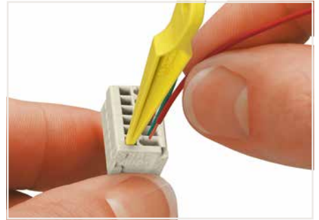
Inserting a conductor via 233-331 Operating Tool. Operation is performed parallel to conductor entry.
