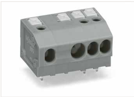
Terminal strips with spacers and enlarged conductor entry (5 mm pin spacing) are available upon request.
