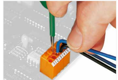
Removing a conductor via push-button.
