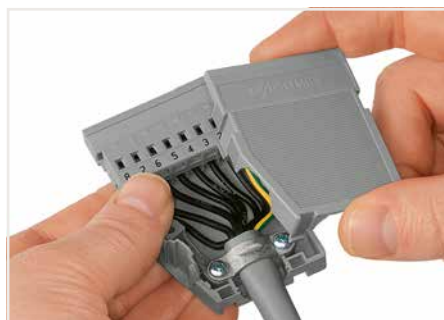
Snapping on a strain relief housing, demonstrated with a female connector with locking levers. Cable exits laterally – strain relief by cable tie (up to a width of 4 mm).
