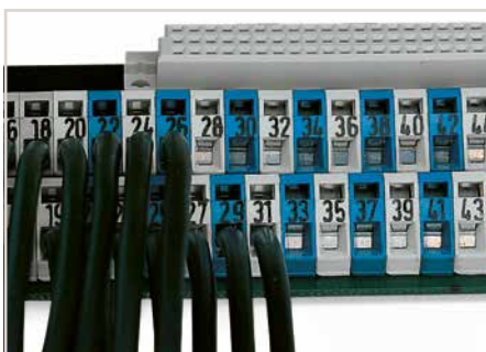
PCB Terminal Strips placed behind each other save space – staggering them by half the pin spacing simplifies subsequent wiring of the first row.
