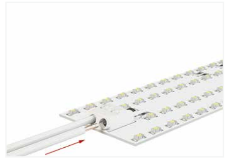
Inserting solid conductors via push-in termination.
