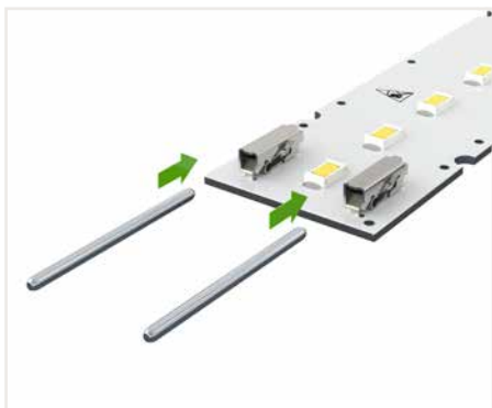
Inserting board-to-board links into the terminal blocks.
