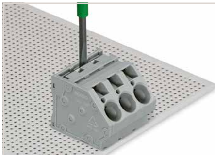
To insert a comb-style jumper bar, push it down using a screwdriver until it hits the backstop – 745 Series.
