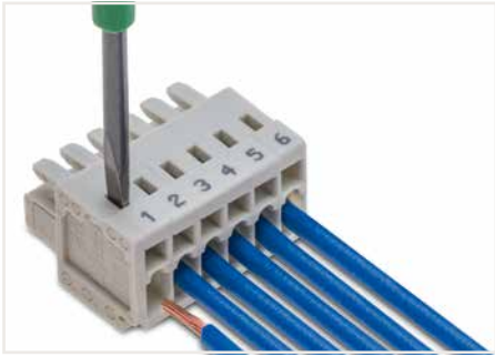
Inserting a conductor via (2.5 x 0.4) mm screwdriver – CAGE CLAMP® actuation perpendicular to conductor entry.
