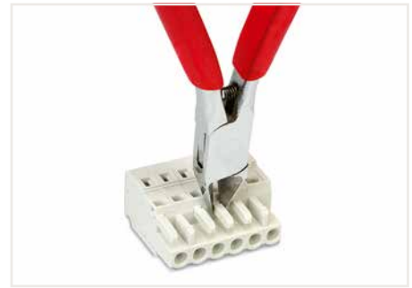
Coding a female connector – removing coding finger(s).
