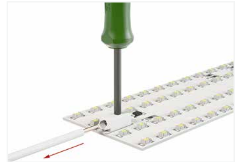
Easy conductor removal, e.g., via operating tool (Item No. 206-859) or "twist & pull" (max. 10 x, no reconnection of smaller conductors possible)
