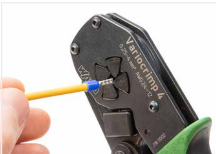
Insert the ferruled conductor into the crimping station.
