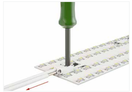
Insert/remove fine-stranded conductors by lightly pressing on push-button, e.g., via optional operating tool (206-860).
