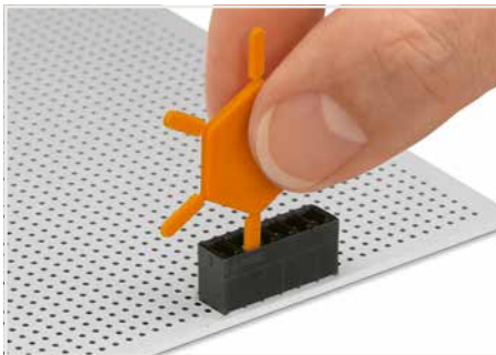
Coding a male header via coding pins.
