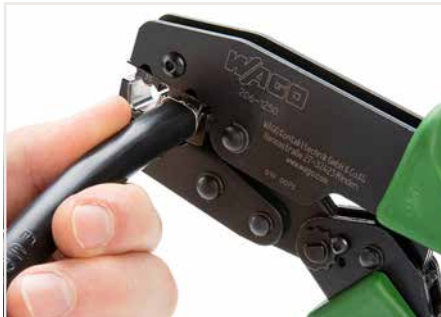
Squeeze handles until ratchet mechanism is released.
