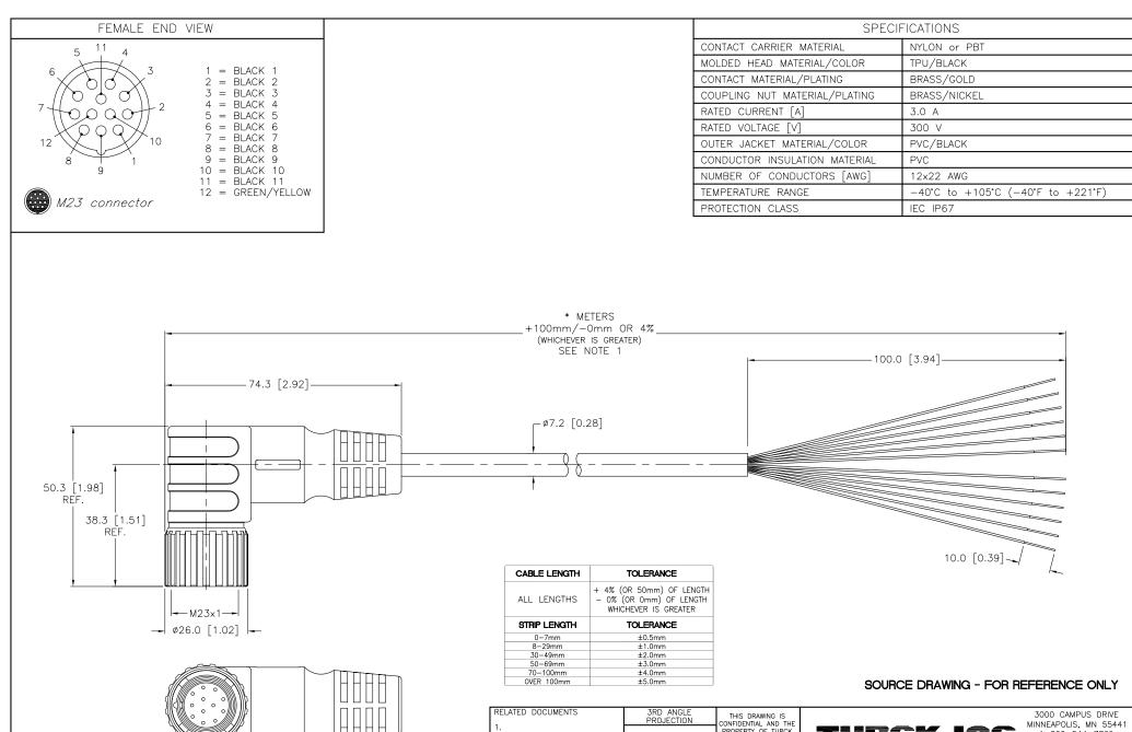
1. "\*" INDICATES CABLE LENGTH IN METERS. CONTACT TURCK TO ORDER SPECIFIC LENGTHS.
