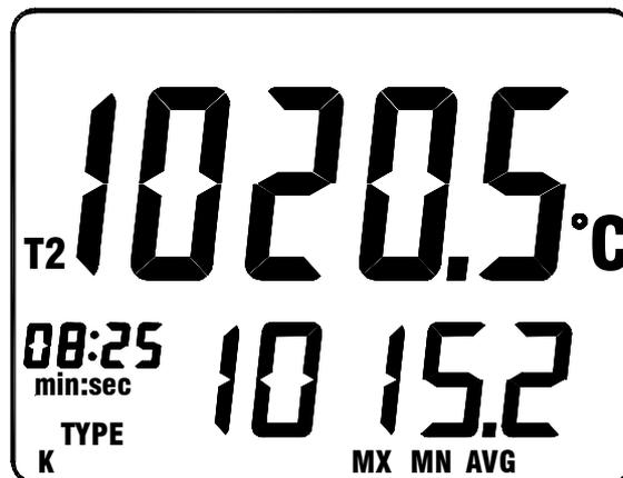
T2 present reading + T2 Maximum reading plus elapsed time + T2 Minimum reading plus elapsed time + T2 Averaging reading plus averaging time.
