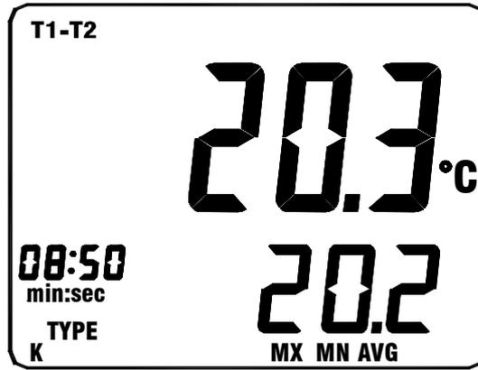
T1-T2 present reading + T1-T2 Maximum reading plus elapsed time + T1-T2 Minimum reading plus elapsed time + T1-T2 Averaging reading plus averaging time.
