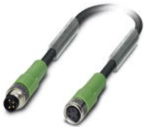
Sensor/Actuator cable, 4-position, PUR halogen-free, black-gray RAL 7021, Plug straight M8, on Socket straight M8, Cable length: 0.3 m
