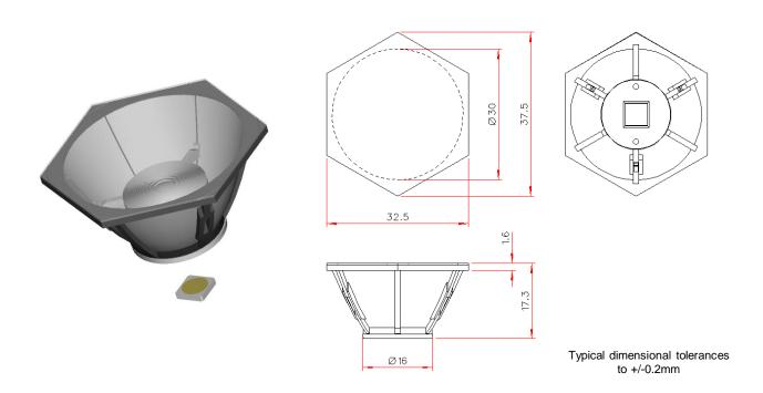
In order to determine if the particular beam properties and performance of this optic are suitable for your application with your chosen LED type, POL suggests that you obtain samples from POL or their distributors for your own product testing, as properties may vary with different LED types.
