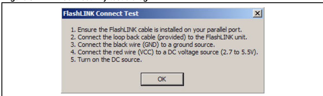
Figure 37. Link connectivity test dialog
