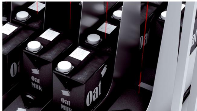
Using the “Two independent switching points” mode, standing and lying objects can be detected and distinguished from one another.
