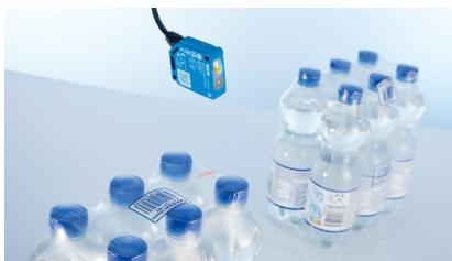
For uneven, shiny and reflective objects, the TwinEye technology® with two receivers of the WTS12 offers high operational safety. Background influences such as reflective high-visibility vests do not interfere with the sensor.
