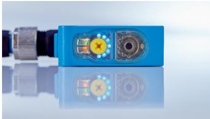
Fast parameterization of photoelectric sensors thanks to Teach-Turn control element for commissioning and fine adjustment.
