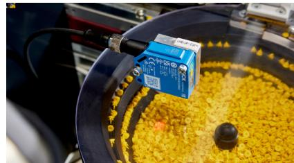
Thanks to foreground suppression, the sensors reliably detect flat, poorly remitting, reflective, and uneven objects.
