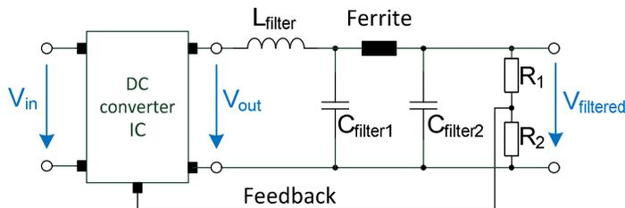
Figure 2: Inclusion of the output filter into the control loop
