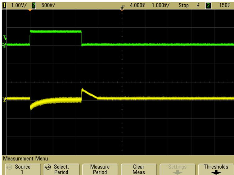
**Figure 4: Transient response of a stabilized switching regulator**
