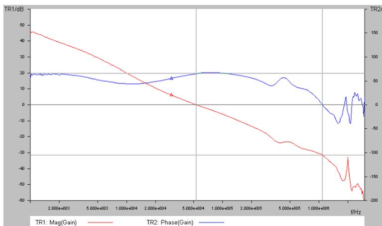
Figure 3: Bode plot of a stabilized switching regulator
