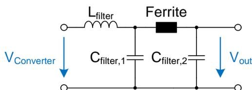
Figure 1: Two-stage output filter
