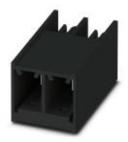
Header, nominal current: 41 A, rated voltage (III/2): 630 V, number of positions: 2, pitch: 7.62 mm, color: black, contact surface: Tin
