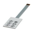
Membrane keypad for BC 107,6 and BC 161,6, self-adhesive, conductive silver technology, 6 keys, 2 colors, 7-pos. terminal lug, pitch: 1.0 mm, customizable in the online configurator
