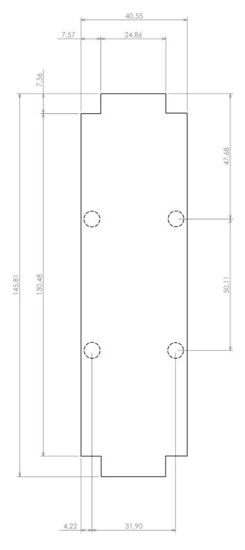
Dashed line shows outline of the mounting boss under PCB board Recommended mounting holes diameter ø3,5mm All dimensions are given within +/-0,5mm tolerance
