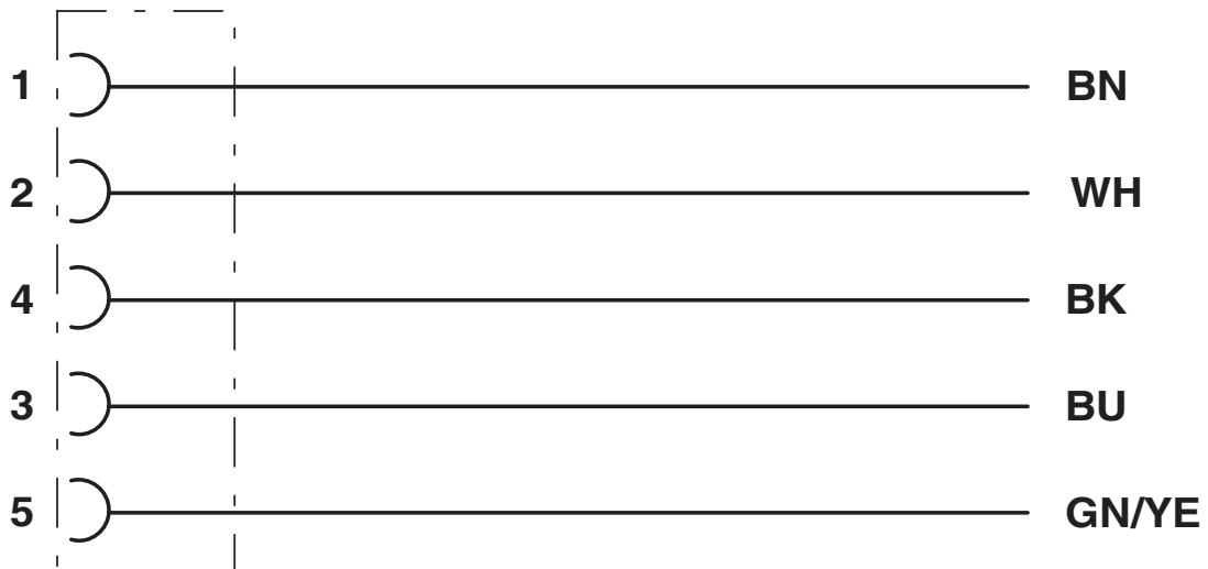
Contact assignment of the M12 sockets
