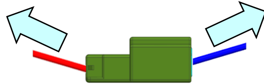
Fig.10-3-5 Condition wires are bent excessively or tension is added
