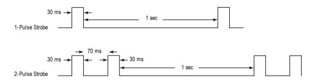
Figure 1. Timing diagram for 1 pulse or 2 pulses
