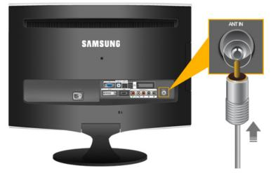
1. Connect the CATV cable or TV antenna cable to the "ANT IN" port on the rear side of the monitor.
