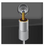
Oconnect the CATV cable or TV antenna cable to the "ANT IN" port on the rear side of the product. Make sure to use a TV antenna cable (sold separately) as the antenna cable.
