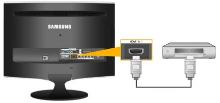
a. Input devices such as digital DVD are connected to the *HDMI IN* terminal of the monitor using the HDMI cable. When all the connections are completed, connect the power cords for the monitor and DVD(or the device connected to the digital output terminal).
