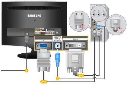
Onnect the power cord for your monitor to the POWER port on the back of the monitor.
