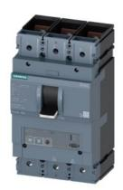
circuit breaker 3VA2 IEC frame 630 breaking capacity class C Icu=110kA @ 415V 3-pole, motor protection ETU350M, LSI, In=400A overload protection Ir=160A...400A short-circuit protection Isd=3...15 x Ir, Ii=15 x In nut keeper kit
