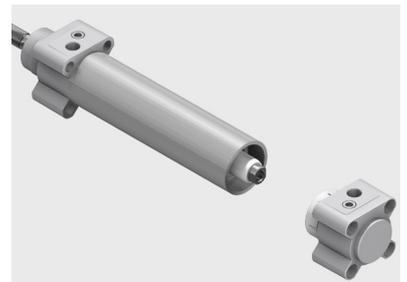
35. Clean the thread of the tie rod to remove the screw locking agent.
