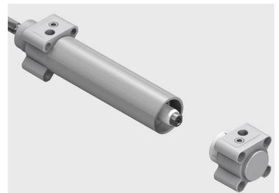
38. Clean the thread of the tie rod to remove the screw locking agent.
